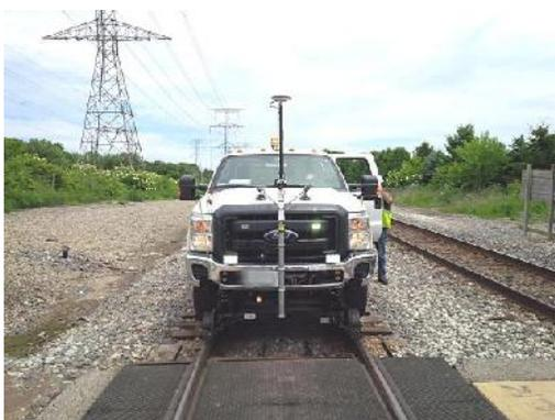
Figure 2. Hi-Rail Vehicle with RTK GPS.
