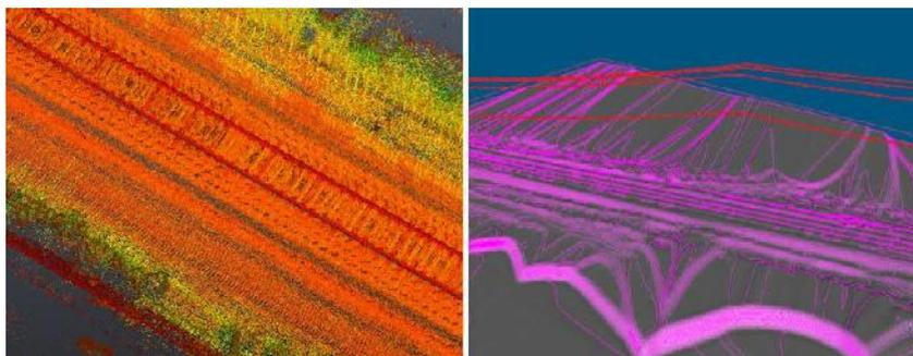
Figure 5. Classified pointcloud data shown by elevation (left). Surface mesh DEM-TIN (right).
